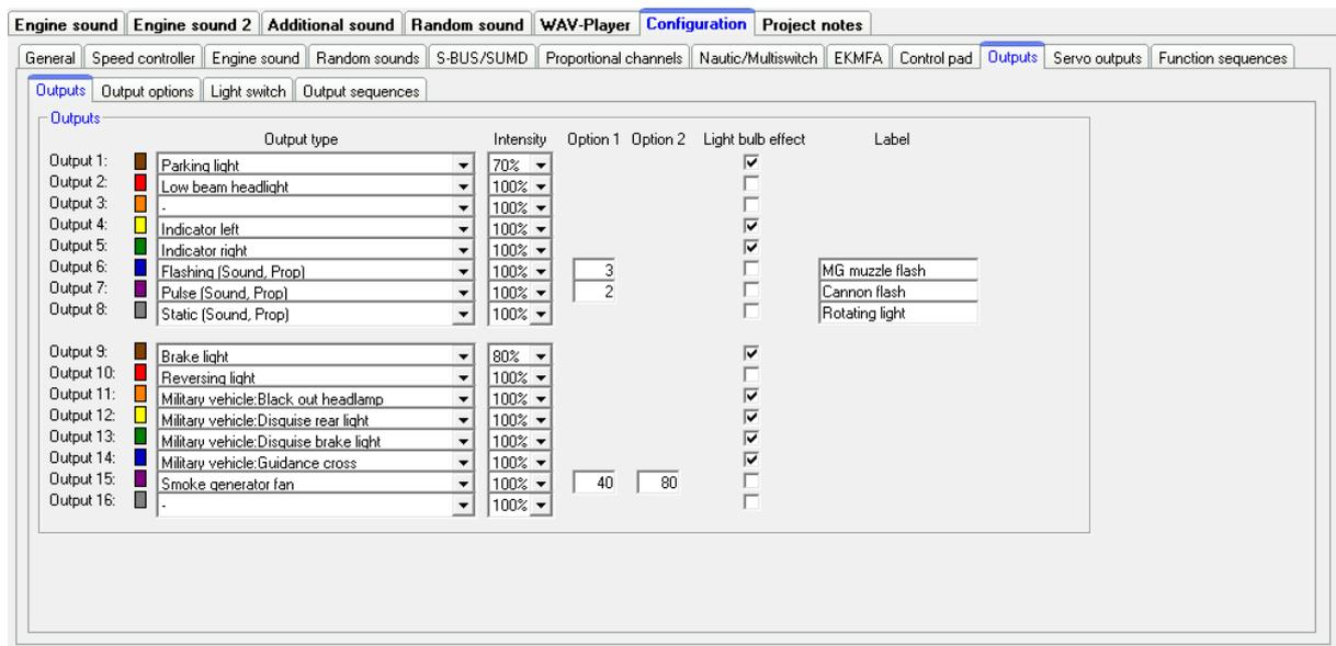
The colored small boxes next to each output indicate the color of the flat ribbon cable that is connected to each output at the SFR-1-D.
