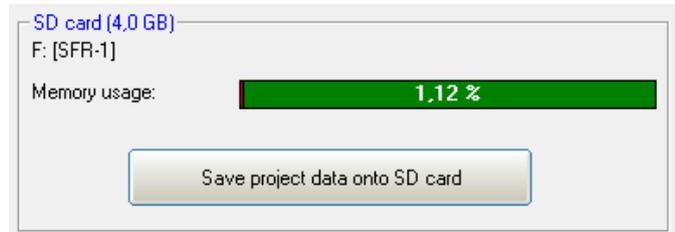
**Memory usage** indicates how much memory on the SD card is in use by the current project.
