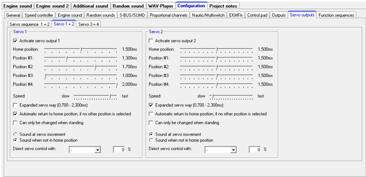
For #1 and #2, e.g. a crane arm will turn slowly to the right and left and at positions #3 and #4 quickly.
