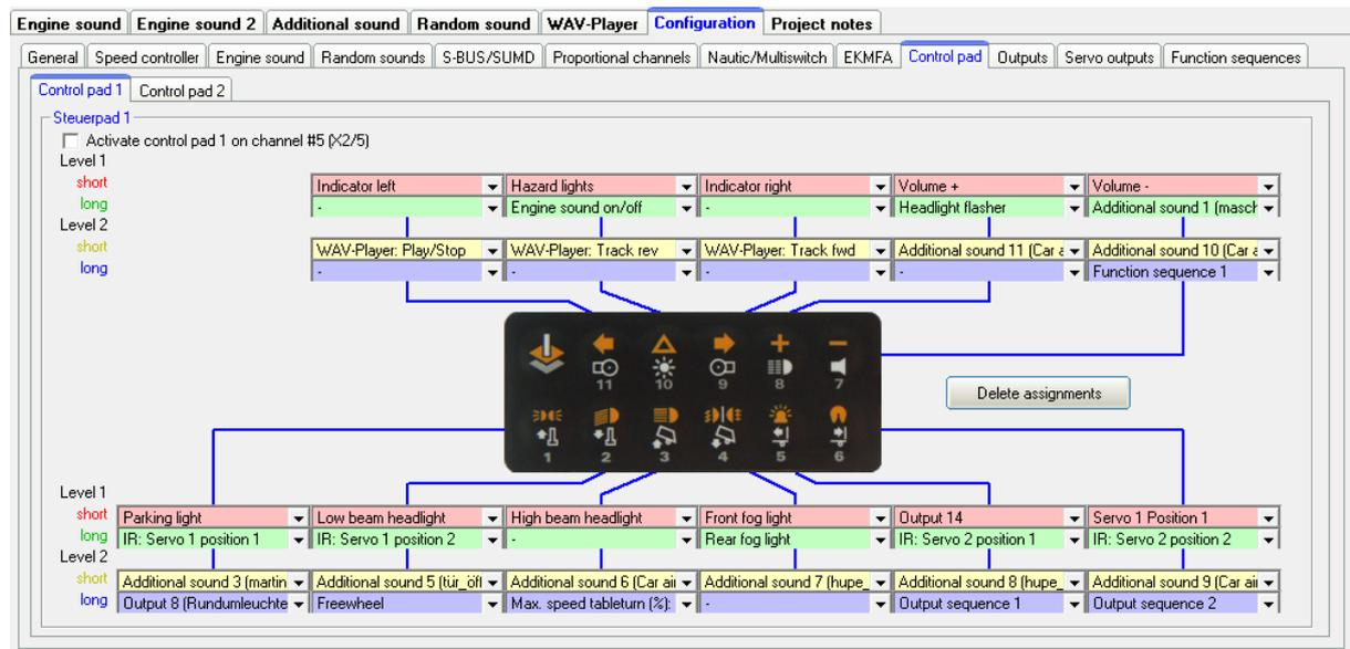
The SFR-1-D can also evaluate the control pads [Light and Sound](#) from the company Kraftwerk. The control pad channel is connected from the receiver output to channel # 5 (X2/5) or channel # 6 (X2/6) of the SFR-1-D.
