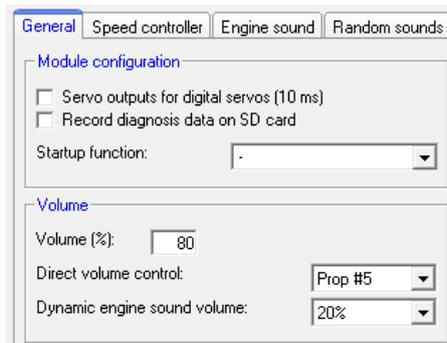
If no potentiometer is connected, the maximum volume, set in the Sound-Teacher (10 – 100 %) at Configuration → General → „Volume (%)” is used.
