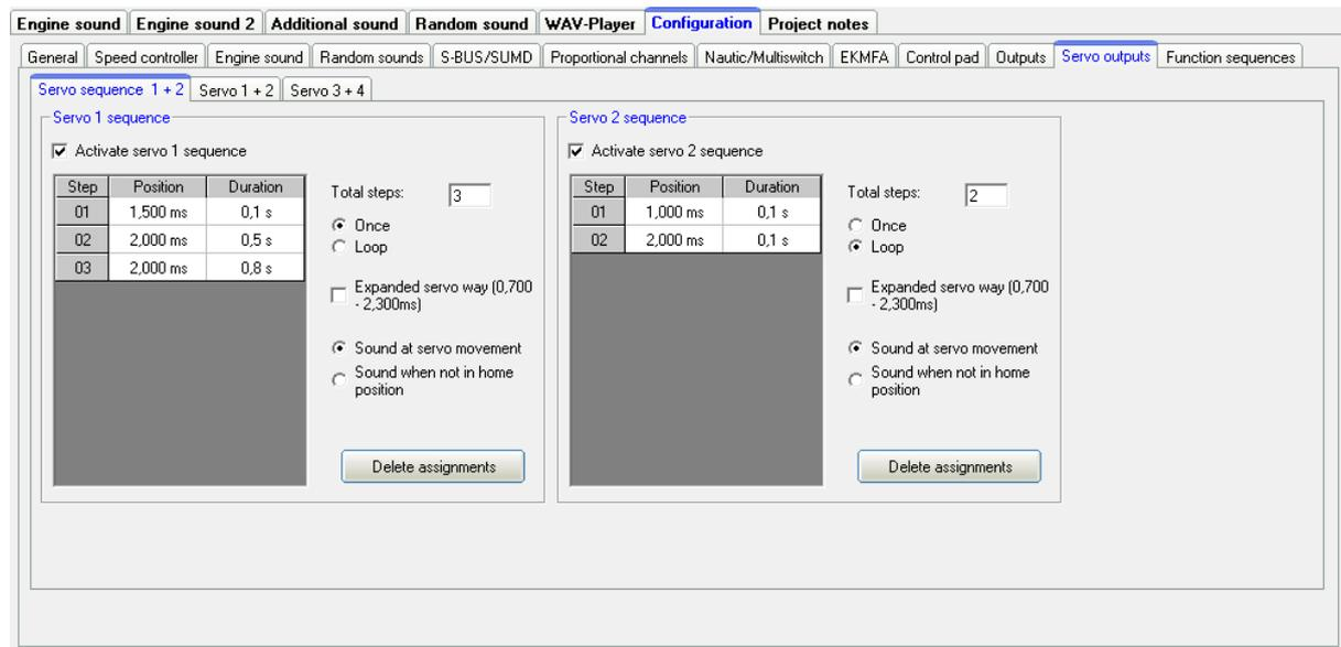
For both servo outputs you can program a time controlled flow sequences. A sequence may consist of up to 10 steps.
