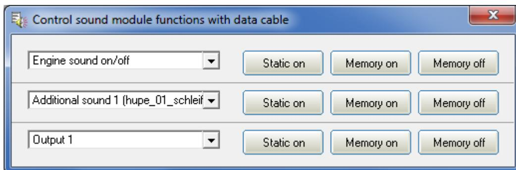
The function “Control SFR-1-D functions with data cable” can be found under menu “Data cable”. With the help of the data cable K-USB-2, all functions can be controlled directly from the PC and not only via the remote control. This can be very helpful for tests without transmitter.
