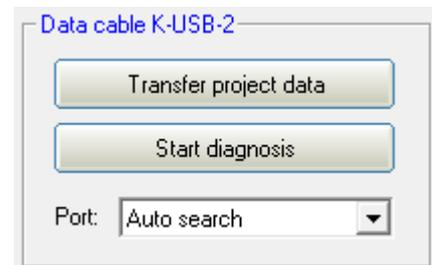
Transferring sounds with the data cable K-USB-2 takes a few minutes! A sound with a length of 10 seconds takes about 15 - 45 seconds (depending on the transmission speed) until it is transferred. Very long songs and large, new projects are only restrictively recommended to be transferred with the data cable.
