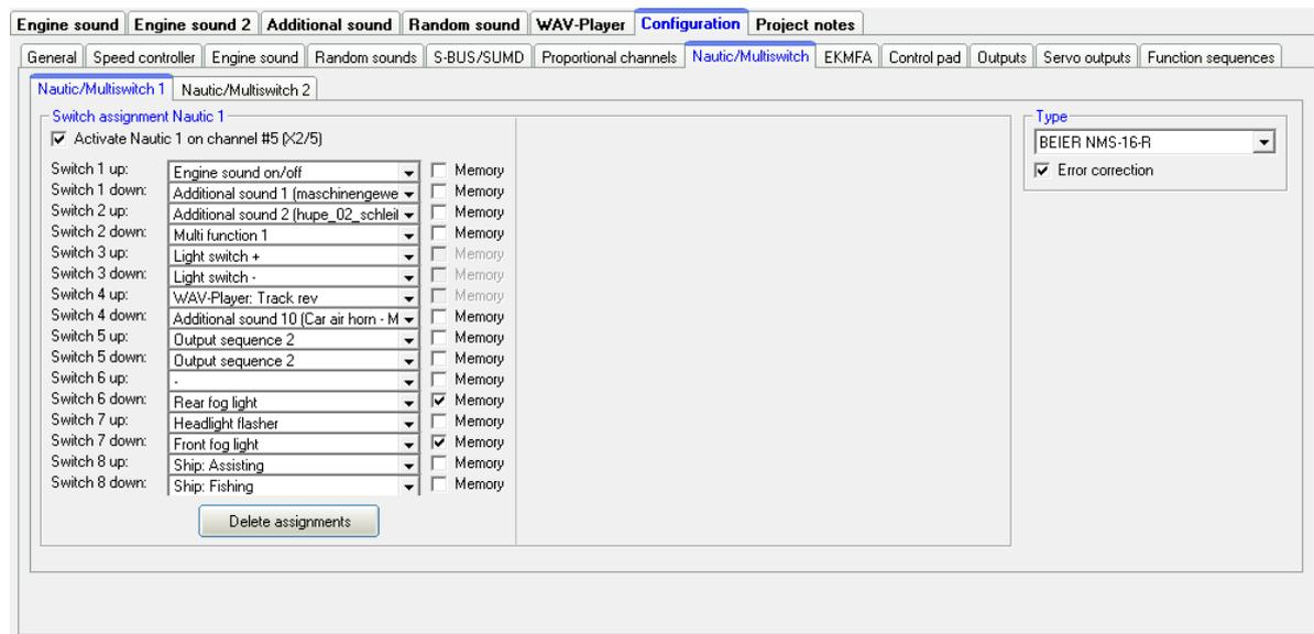
If you want to use the nautic mode 1 or 2, you will first have to activate it here and connect the SFR-1-D prop. channel #5 (X2/5) or #6 (X2/6) to the receiver channel.
